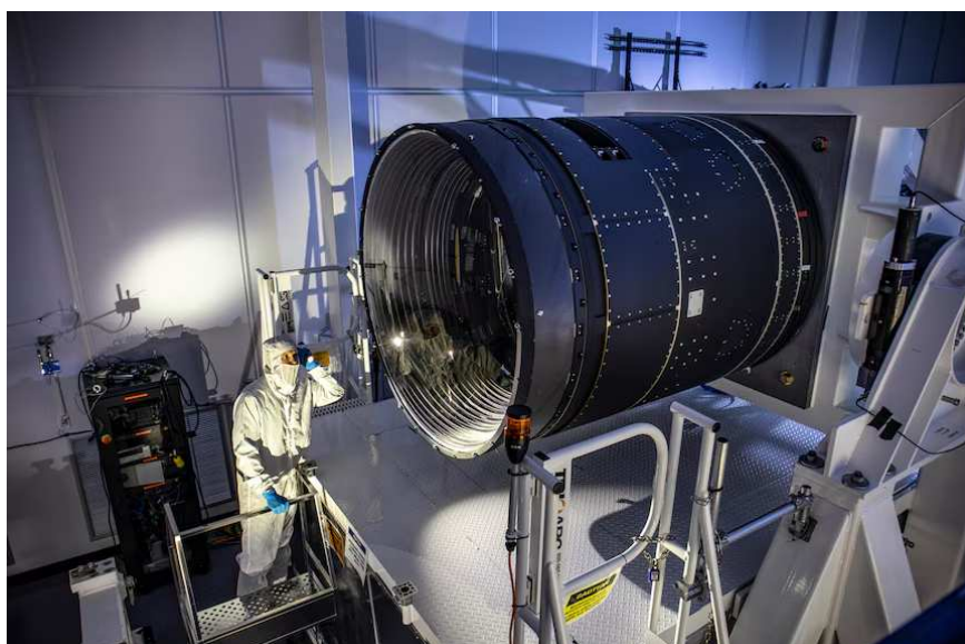
The 3,200-megapixel camera will be connected to the Simonyi Survey Telescope inside the observatory. (Supplied: Jacqueline Ramseyer Orrell/SLAC National Accelerator Laboratory)
